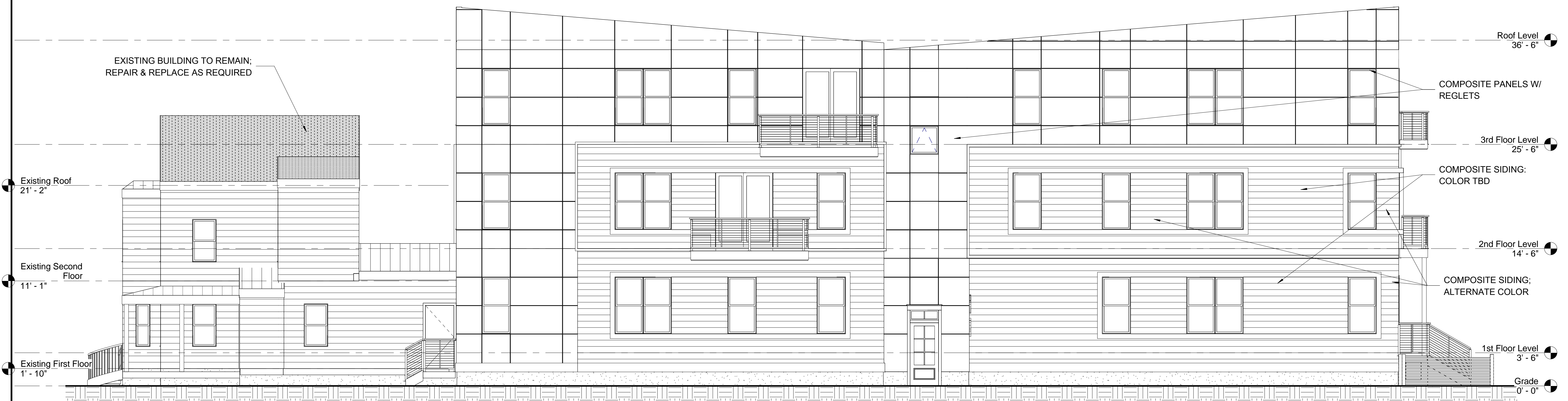
② Left Side Elevation 3/16" = 1'-0"
