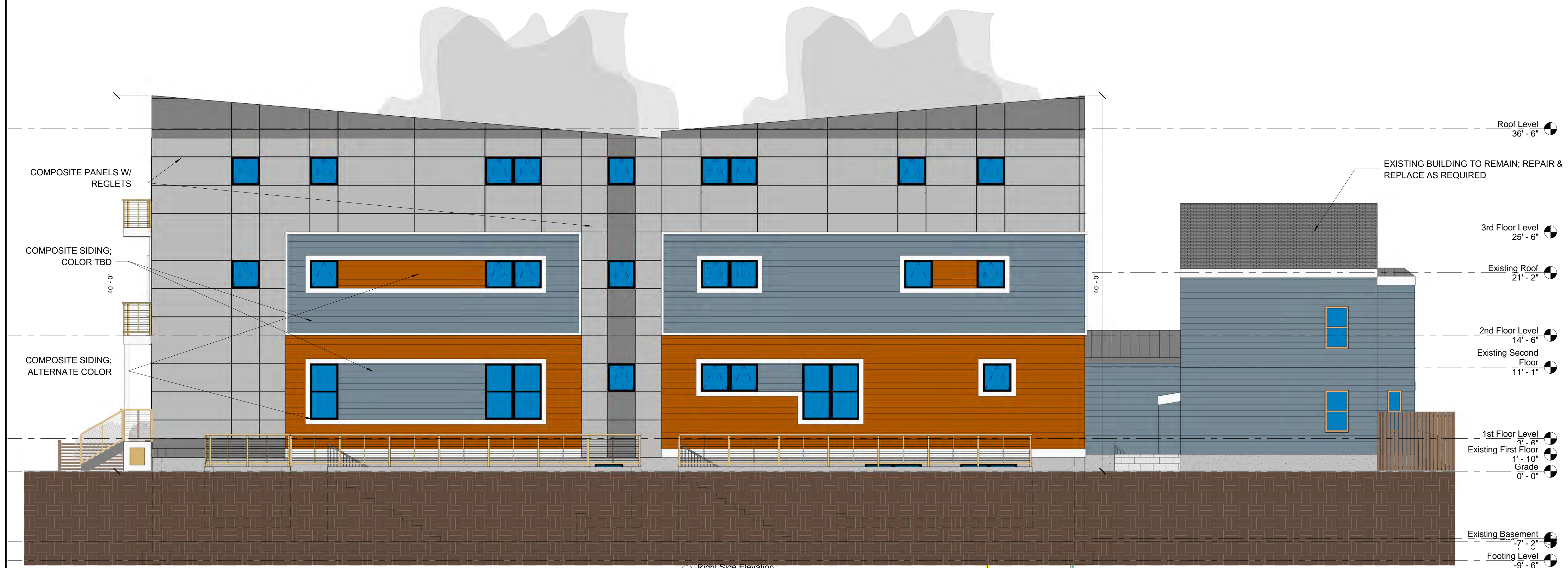
② Right Side Elevation 3/16" = 1'-0"
